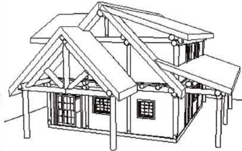
Post and Beam Construction
